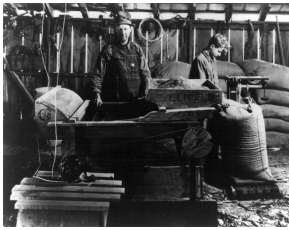
Figure 2. Electricity also brought new technology to the farm. Many farmers built their own machinery, such as this electric-powered feed mixer.
